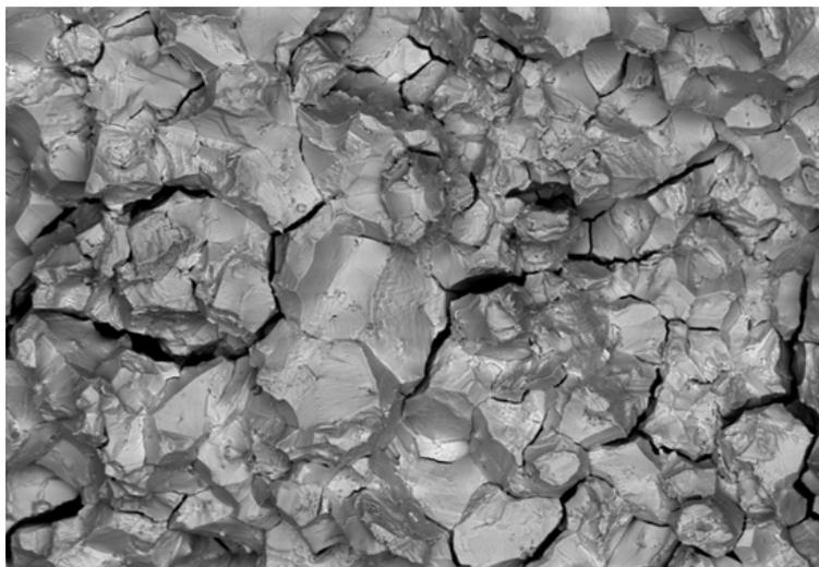
*SEM image of the surface of a fractured bolt showing an intergranular fracture mode; this particular sample failed by SCC.*
