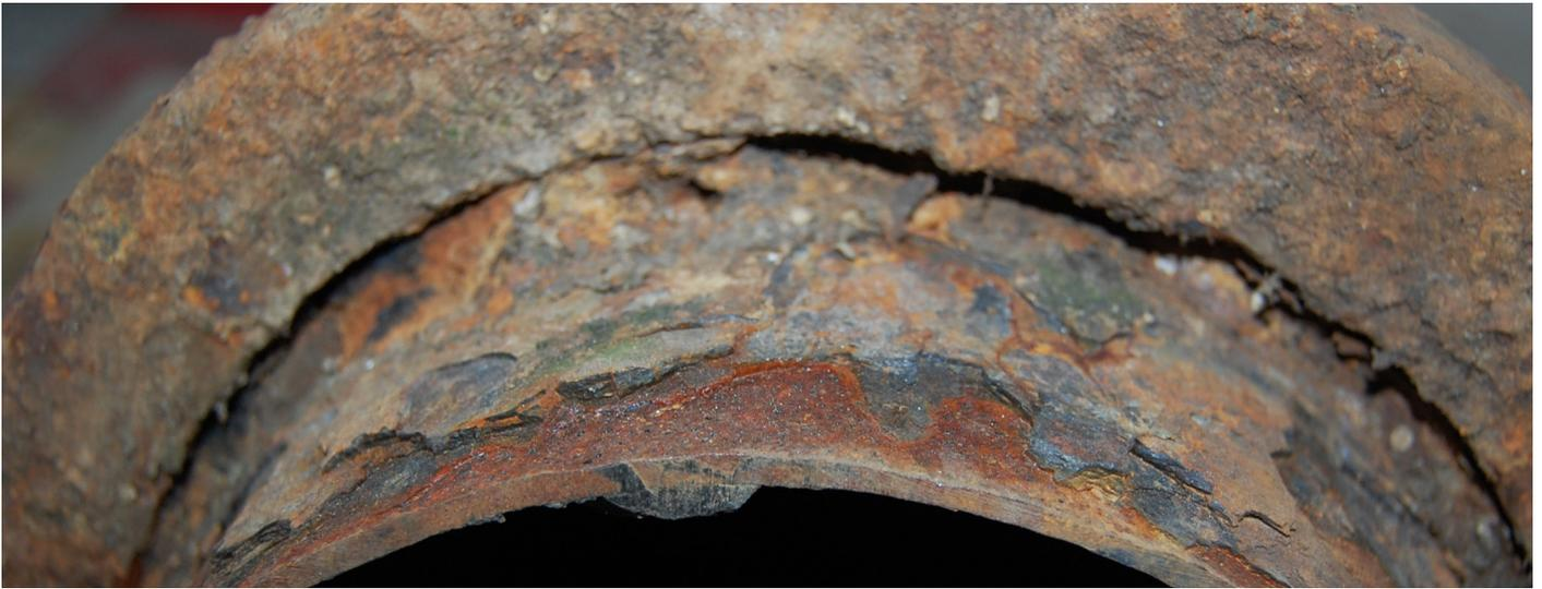
The image below shows uniform corrosion scale on a copper water pipe. Some variation in the thickness can be seen as shown by the colour variation. This form of scale generally builds up in the early stages of exposure to the water, but which then forms a protective layer reducing the corrosion rate to a negligible level.
