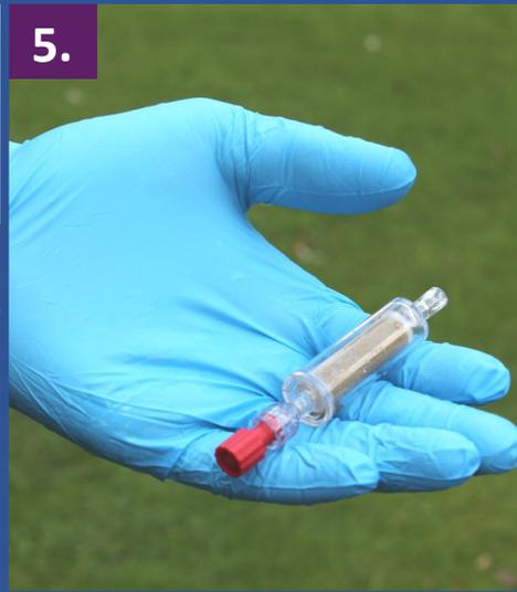
Screw one red cap tightly on to the thick end of the filter unit.
