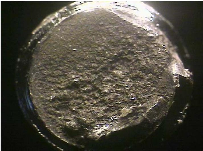
This fractured wheel-spoke reveals fatigue marks but they could easily be destroyed by dropping or rubbing in transit, as it is only 3mm diameter. This makes packaging an important part of the examination.
