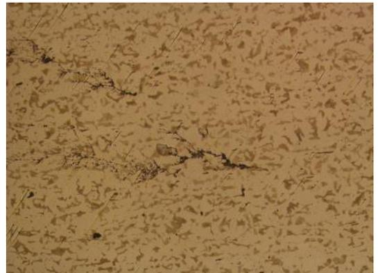
A microstructure of ferrite and pearlite. Fingers of slag date the steel to probably between the wars.
