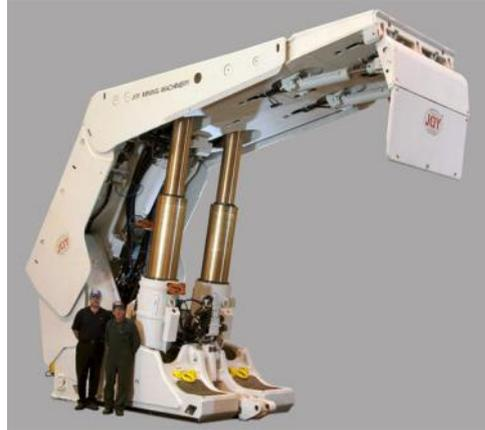
These roof supports are pretty impressive structures. A row of these form a 'long-wall' along the coal face, and as the cutter flies along its track, alternate roof supports retract and walk forwards, pushing the cutter track to its new position.
